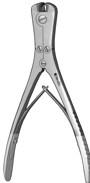
P.I. FLUSH WIRE CUTTER KM 46-631 7" front and side cutting with carbide inserts, double action maximum capacity .062" (1.6mm)
